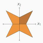
• Best optimal value  $\underline{f}$  of min  $\mathbf{c}^T x : \mathbf{A} x \leq \mathbf{b}, x \geq 0$ Non-negative variables  $\Rightarrow$  objective vector  $\underline{c}$ Largest feasible set:  $\underline{A} x \leq \overline{b}, x \geq 0$
